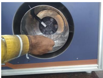
STEP – 8 : Replace the inner chamber & grill plate
