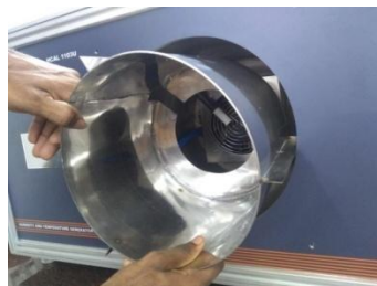
STEP – 5 : Remove the Inner Chamber
