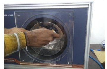
STEP – 9 : Replace the Front acrylic door and close using 4 knobs
