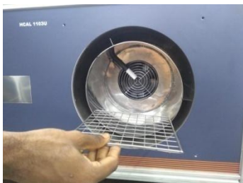
STEP – 4 : Remove the Inner grill plate
