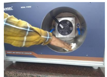
STEP – 6 : Clean chamber surface thoroughly using tissue paper
